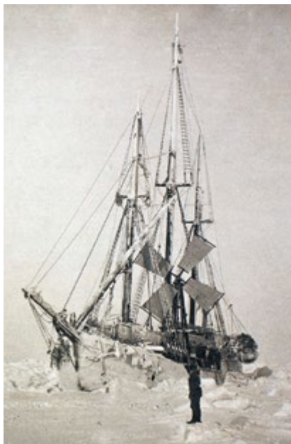
Fram ship in March 1894. Wind turbine of the electric generator is clearly visible
