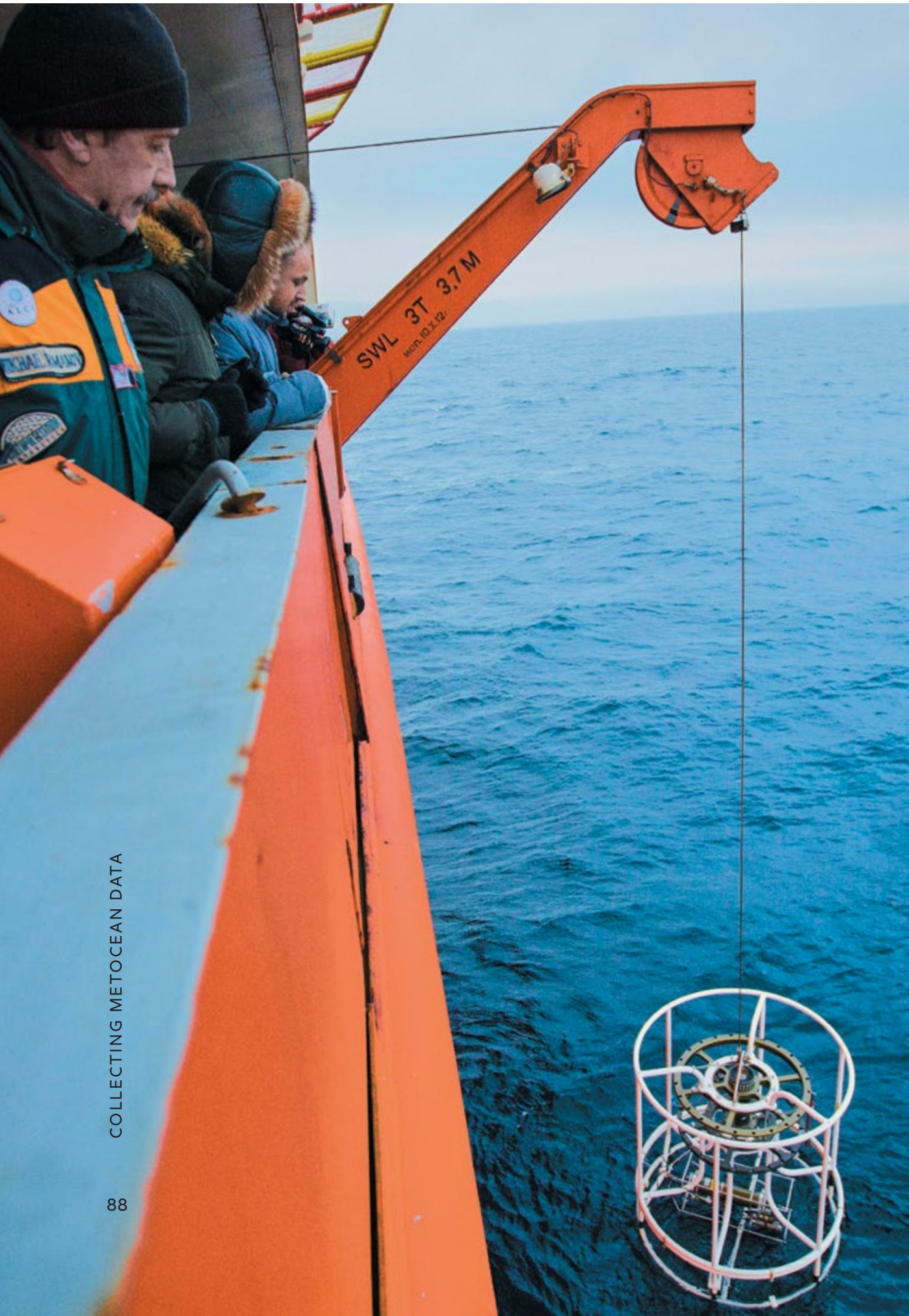
Study of the thermohaline structure, descending a rosette sampler with a bathometer
