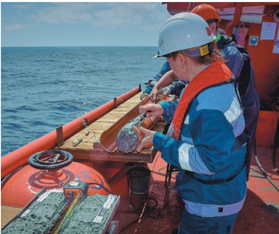
Geotechnical studies. Core extraction from a coring tube
