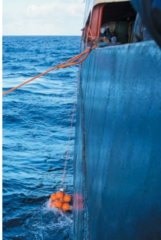
Deployment of a submerged autonomous buoy station (SABS), Chukotka-Summer 2015
