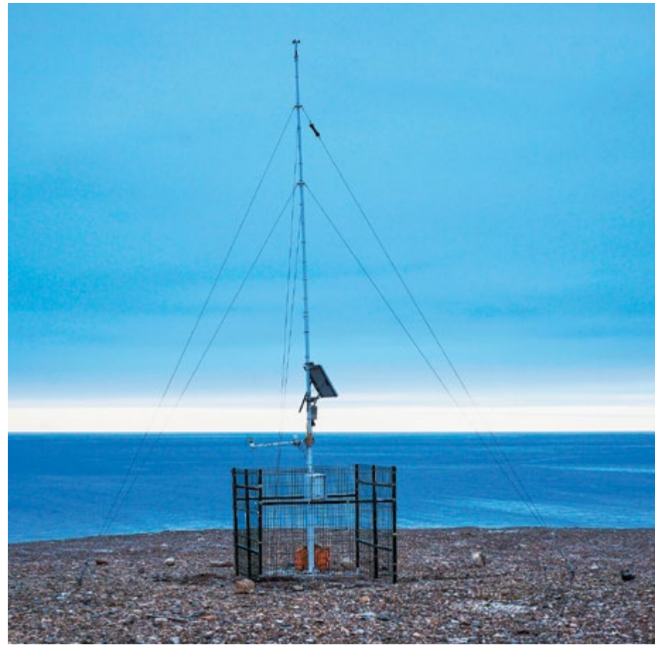
An automatic weather station fenced with bear protection mesh
